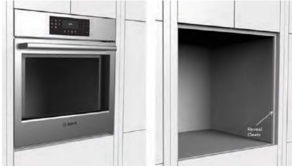
Example Flush Install
